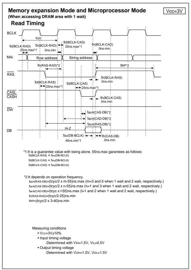
Figure 1.28.21. Vcc=3V timing diagram (7)
