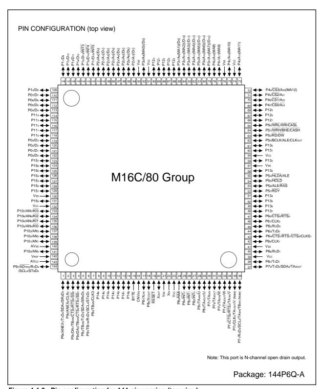
Figure 1.1.3. Pin configuration for 144-pin version (top view)
