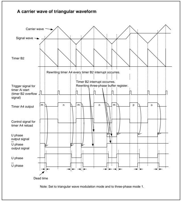
Figure 1.15.7. Timing chart of operation (2)
