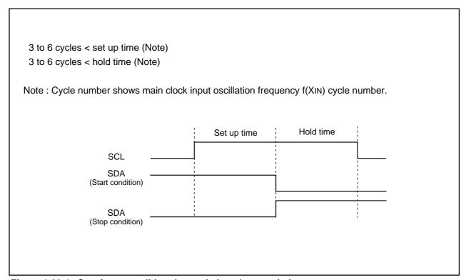
Figure 1.20.4. Start/stop condition detect timing characteristics
