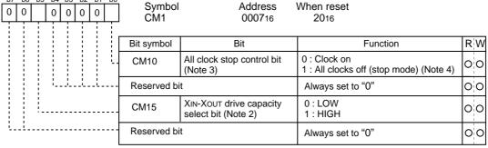
Note 1: Set bit 0 of the protect register (address 000A16) to "1" before writing to this register.
