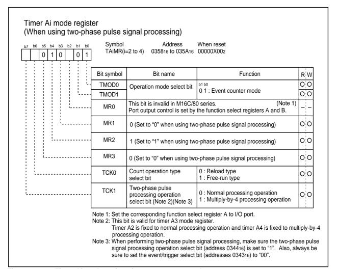
Figure 1.13.7. Timer Ai mode register in event counter mode
