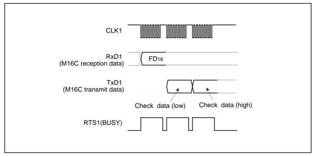
Figure 1.31.19. Timing for the read check data
