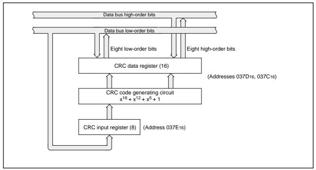
Figure 1.23.1. Block diagram of CRC circuit
