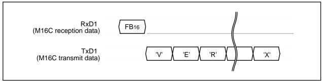
Figure 1.31.35. Timing for version information output
