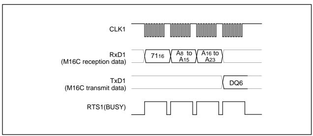
Figure 1.31.11. Timing for reading lock bit status
