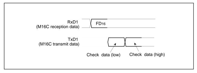
Figure 1.31.39. Timing for the read check data
