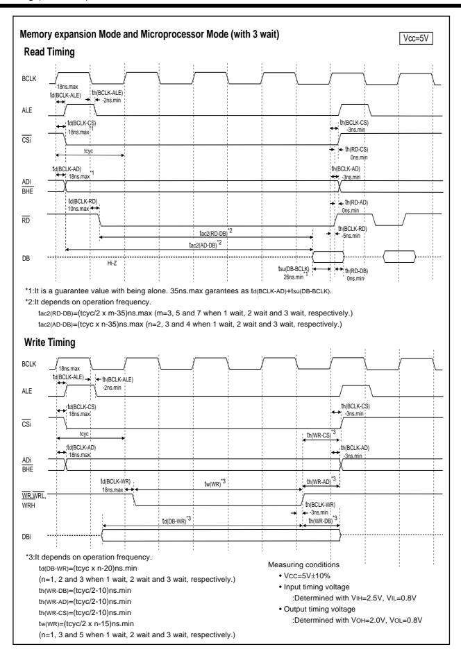
Figure 1.28.5. Vcc=5V timing diagram (4)
