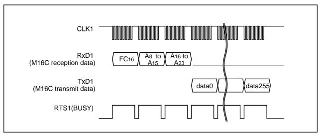
Figure 1.31.16. Timing for boot ROM area output
