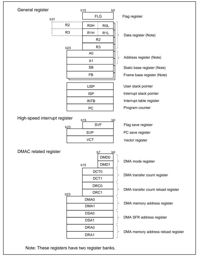
Figure 1.3.1. Central processing unit register
