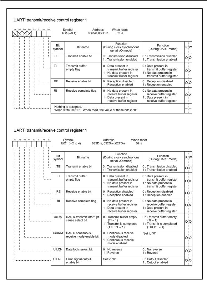
Figure 1.16.9. Serial I/O-related registers (5)
