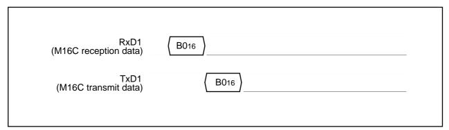
Figure 1.31.40. Timing of baud rate 9600
