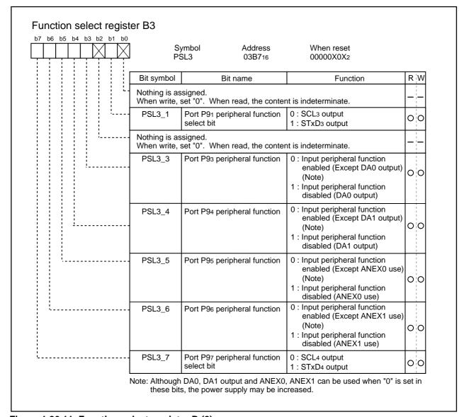
Figure 1.26.11. Function select register B (2)
