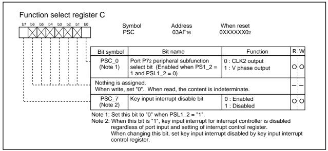
Figure 1.26.12. Function select register C
