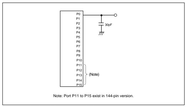
Figure 1.28.1. Port P0 to P15 measurement circuit
