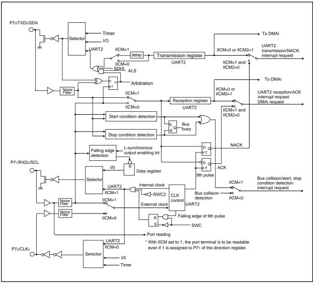
Figure 1.20.2. Functional block diagram for I<sup>2</sup>C mode
