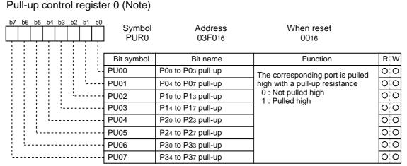
Note: Since P0 to P5 operate as the bus in memory expansion mode and microprocessor mode, do not set the pull-up control register. However, it is possible to select pull-up resistance presence to the usable port as I/O port by setting.
