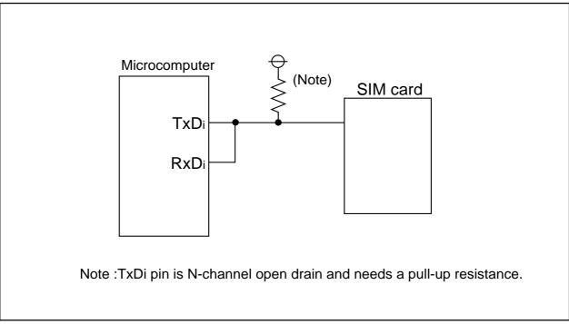
Figure 1.19.4. Connecting the SIM interface
