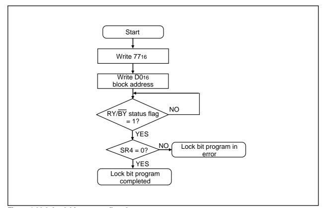
Figure 1.30.6. Lock bit program flowchart
