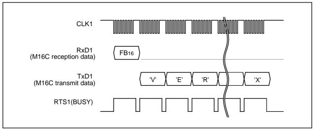
Figure 1.31.15. Timing for version information output
