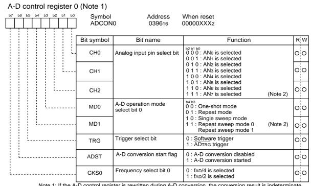
Note 1: If the A-D control register is rewritten during A-D conversion, the conversion result is indeterminate. Note 2: When changing A-D operation mode, set analog input pin again.
