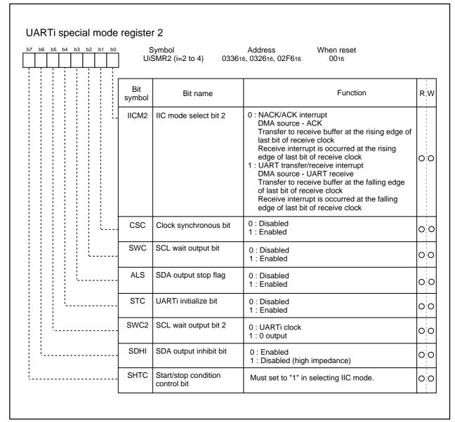
Figure 1.16.11. Serial I/O-related registers (7)
