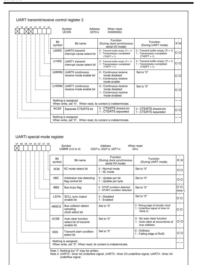
Figure 1.16.10. Serial I/O-related registers (6)
