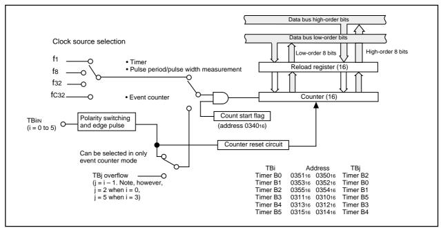
Figure 1.14.1. Block diagram of timer B
