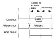
Note: These examples show the address bus and chip select signal for two consecutive cycles. By combining these examples, chip select signal can be extended beyond two cycles.
