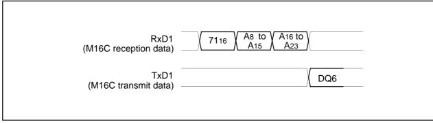
Figure 1.31.31. Timing for reading lock bit status
