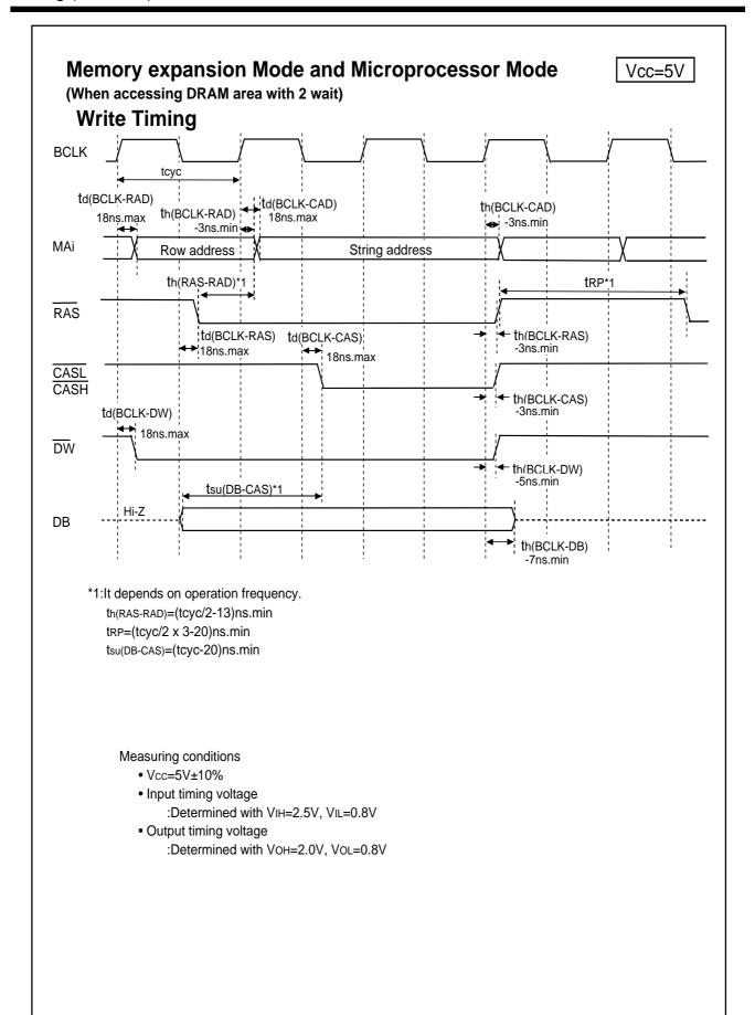
Figure 1.28.11. Vcc=5V timing diagram (10)
