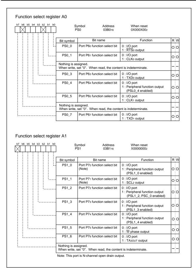
Figure 1.26.8. Function select register A (1)
