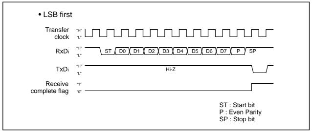
Figure 1.19.2. Output timing of the parity error signal
