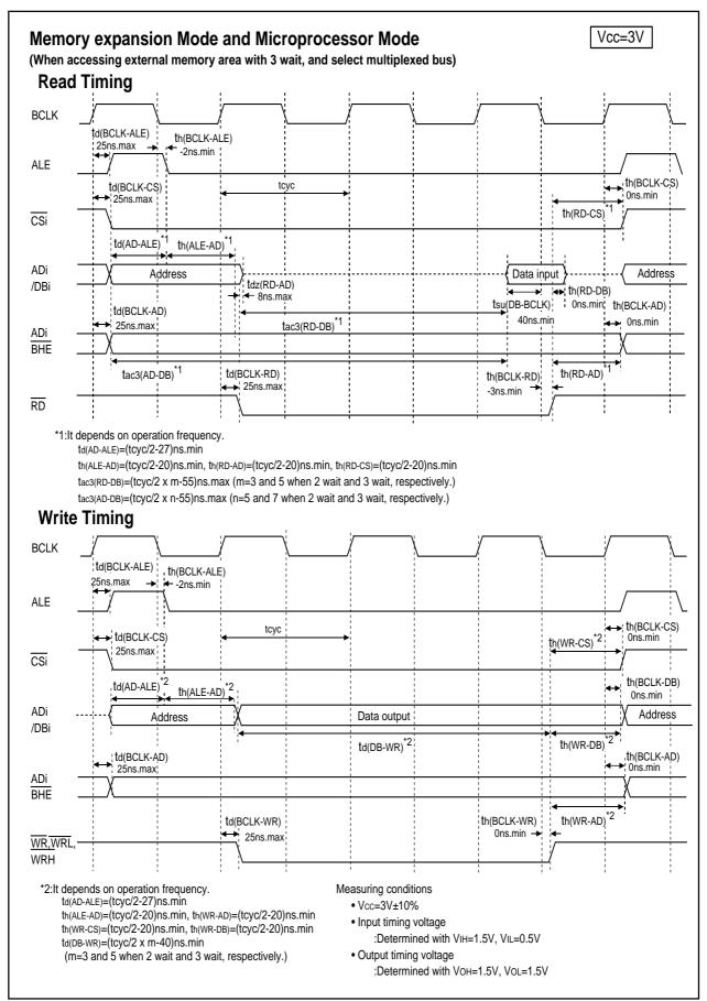
Figure 1.28.20. Vcc=3V timing diagram (6)
