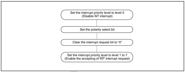
Figure 1.9.12. Switching condition of INT interrupt request
