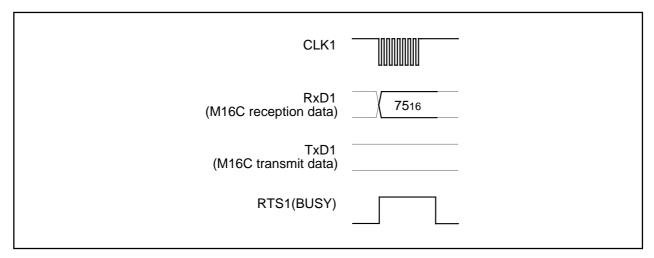
Figure 1.31.13. Timing for disabling the lock bit
