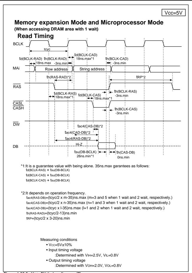
Figure 1.28.8. Vcc=5V timing diagram (7)
