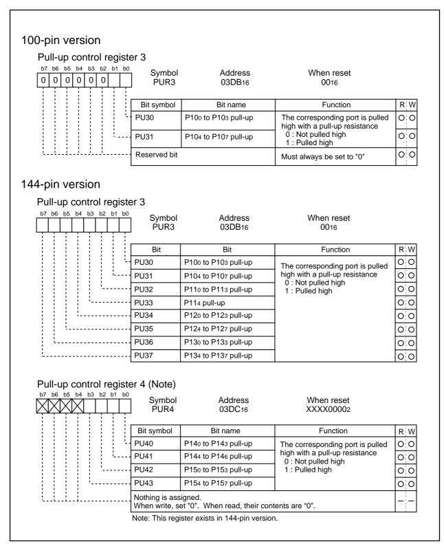
Figure 1.26.14. Pull-up control register (2)
