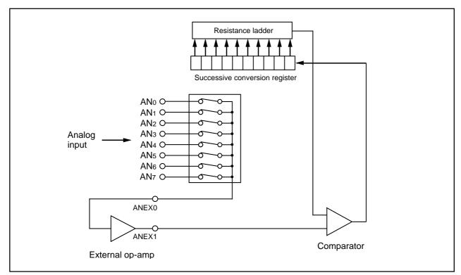
Figure 1.21.9. Example of external op-amp connection mode
