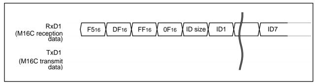
Figure 1.31.37. Timing for the ID check
