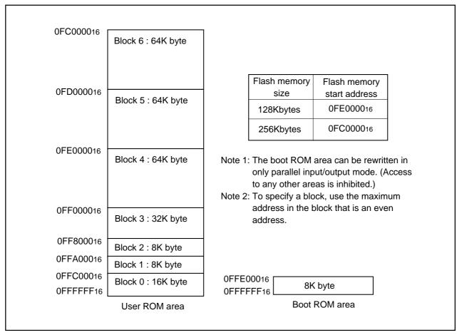
Figure 1.29.3. Block diagram of flash memory version
