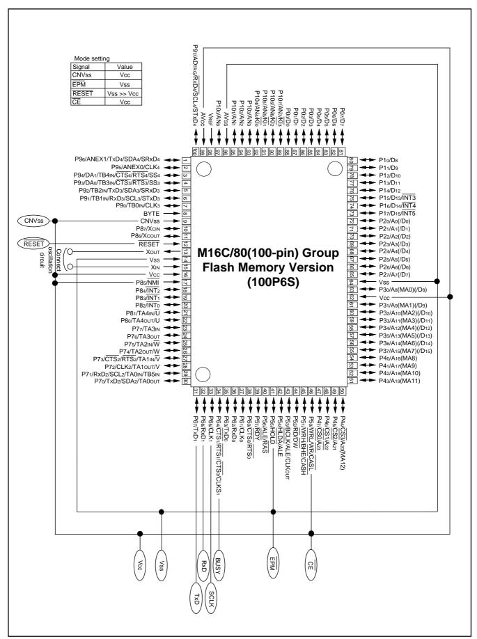
Figure 1.31.1. Pin connections for standard serial I/O mode (1)
