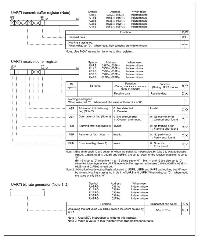
Figure 1.16.5. Serial I/O-related registers (1)
