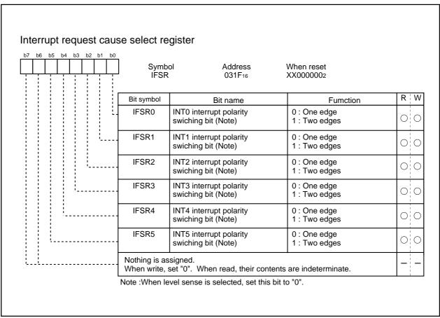
Figure 1.9.9 Interrupt request cause select register
