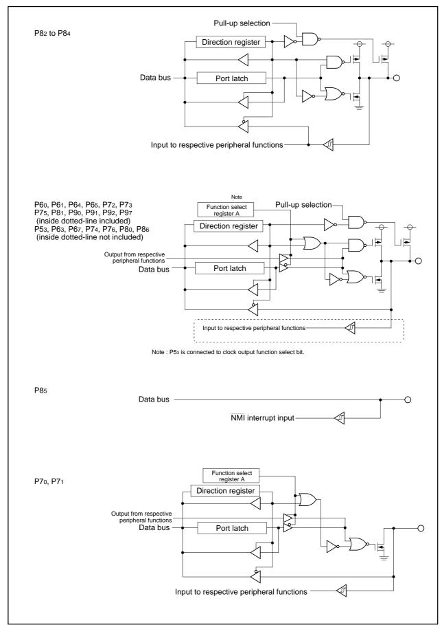
Figure 1.26.2. Programmable I/O ports (2)
