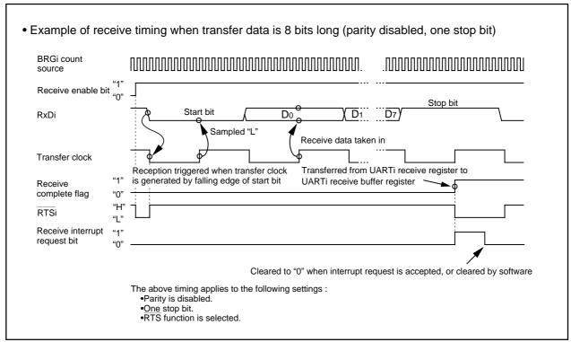
Figure 1.18.3. Typical receive timing in UART mode
