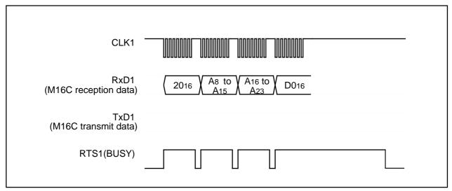
Figure 1.31.8. Timing for block erasing
