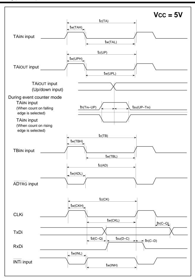
Figure 1.28.13. Vcc=5V timing diagram (12)
