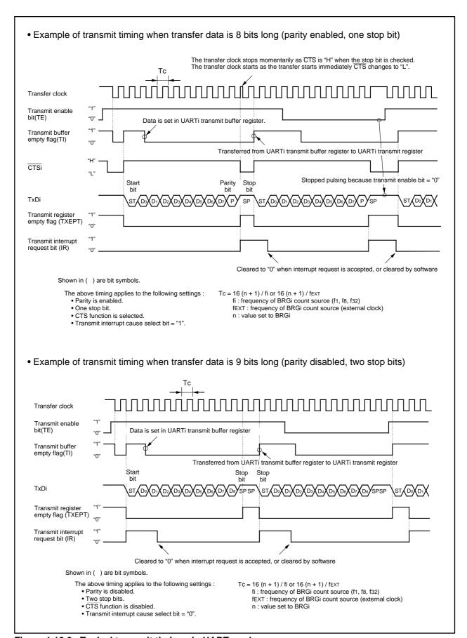
Figure 1.18.2. Typical transmit timings in UART mode
