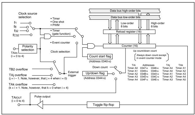
Figure 1.13.1. Block diagram of timer A
