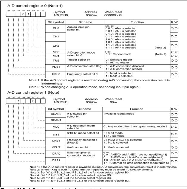
Figure 1.21.5. A-D conversion register in repeat mode
