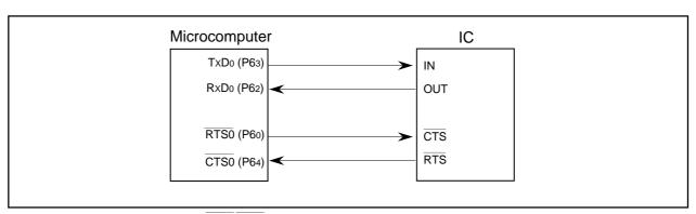
Figure 1.18.4. The separate CTS/RTS pins function usage
