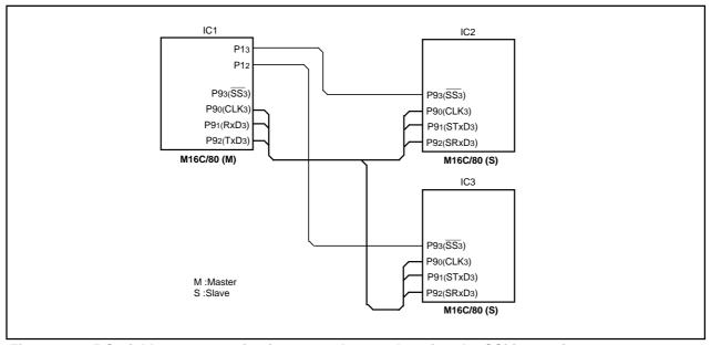
Figure 1.20.5 Serial bus communication control example using the SSi input pins
