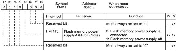
Note: For this bit to be set to "1", the user needs to write a "0" and then a "1" to it in succession. When it is not this procedure, it is not enacted in "1". This is necessary to ensure that no interrupt or DMA transfer will be executed during the interval. Use the control program except in the internal flash memory for write to this bit.
