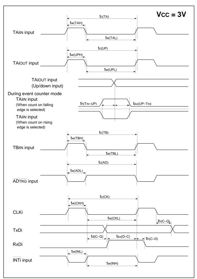
Figure 1.28.26. Vcc=3V timing diagram (12)
