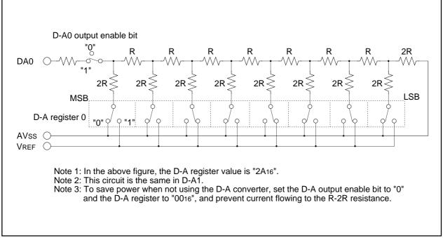
Figure 1.22.3. D-A converter equivalent circuit
