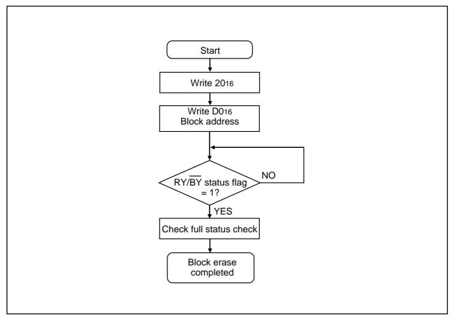
Figure 1.30.5. Block erase flowchart
