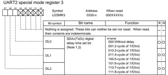
Note 1: These bits are used for SDA2(TxD2) output digital delay when using UART2 for IIC interface. Otherwise, must set to "000".
