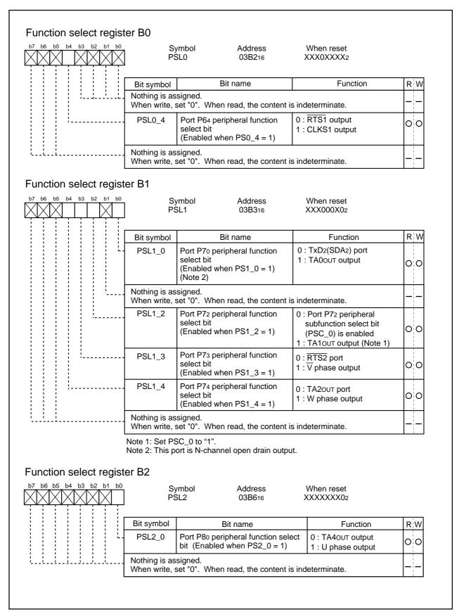
Figure 1.26.10. Function select register B (1)
