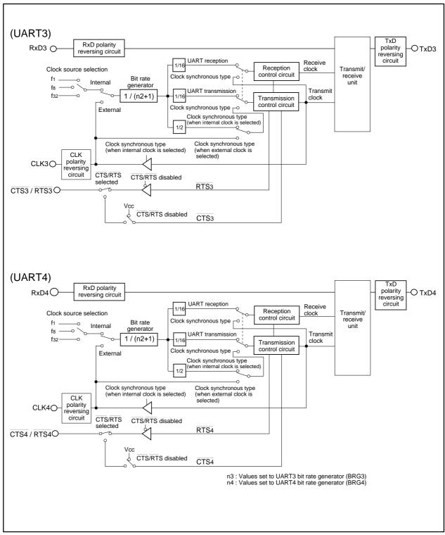
Figure 1.16.2. Block diagram of UARTi (i = 3, 4)
