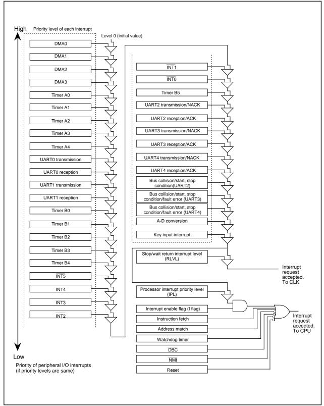
Figure 1.9.8. Interrupt resolution circuit
