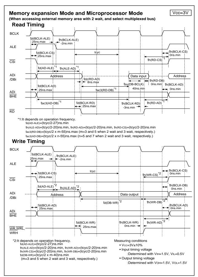
Figure 1.28.19. Vcc=3V timing diagram (5)
