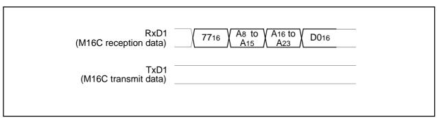
Figure 1.31.30. Timing for the lock bit program
