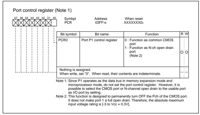
Figure 1.26.15. Port control register
