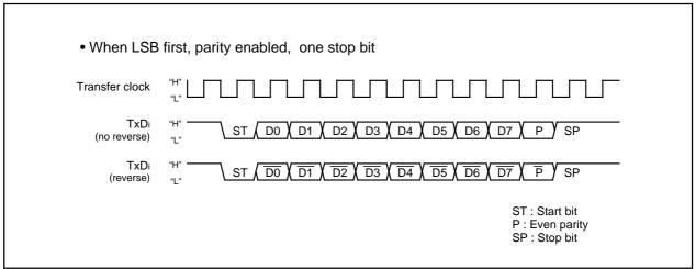
Figure 1.18.5. Timing for switching serial data logic
