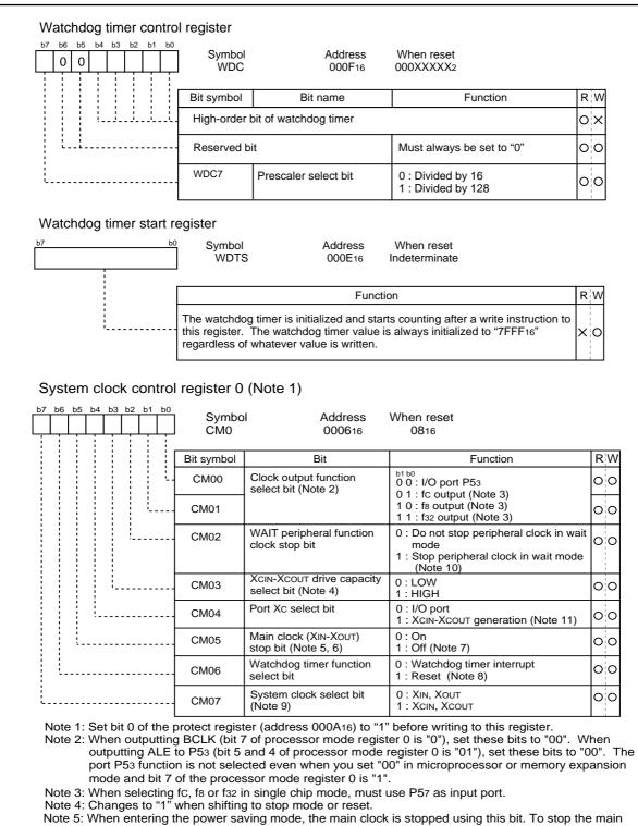
Note 5: When entering the power saving mode, the main clock is stopped using this bit. To stop the main clock, set system clock stop bit (CM07) to "1" while an oscillation of sub clock is stable. Then set this bit to "1".
