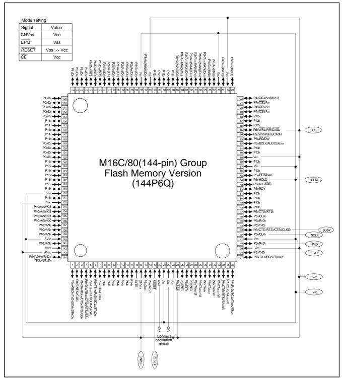
Figure 1.31.3. Pin connections for standard serial I/O mode (3)
