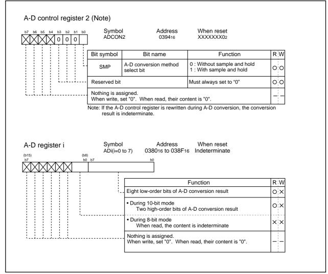
Figure 1.21.3. A-D converter-related registers (2)
