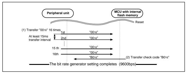
Figure 1.31.23. Peripheral unit and initial communication
