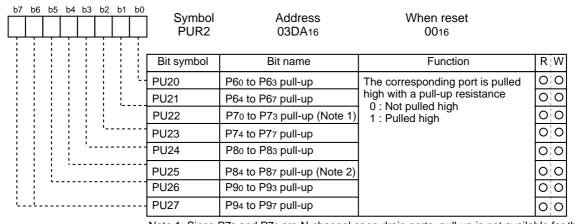
Note 1: Since P70 and P71 are N-channel open drain ports, pull-up is not available for them. Note 2: Except port P85.
