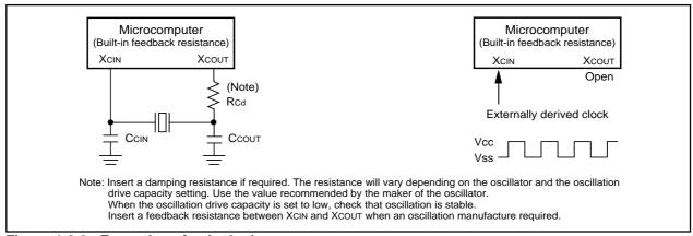
Figure 1.8.2. Examples of sub clock
