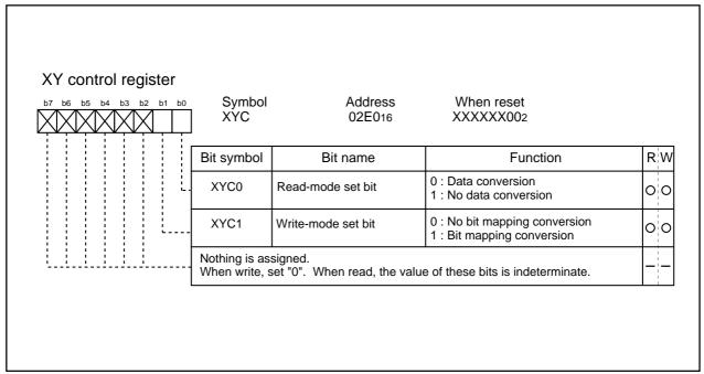
Figure 1.24.1. XY control register
