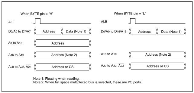
Figure 1.7.3. ALE signal and address/data bus
