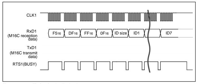
Figure 1.31.17. Timing for the ID check
