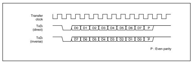
Figure 1.19.3. SIM interface format
