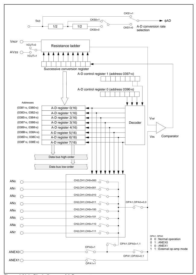
Figure 1.21.1. Block diagram of A-D converter
