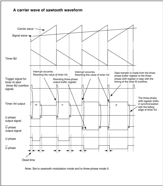
Figure 1.15.9. Timing chart of operation (4)
