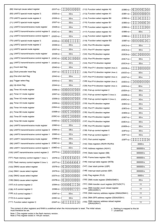
Figure 1.4.4. Device's internal status after a reset is cleared
