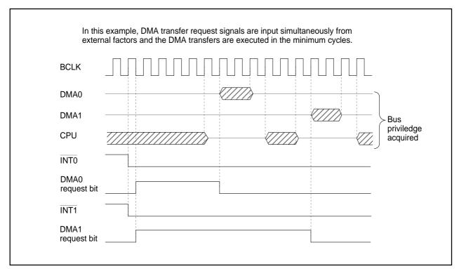
Figure 1.11.7. DMA transfer example by external factors
