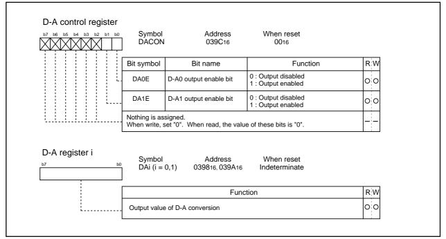
Figure 1.22.2. D-A control register
