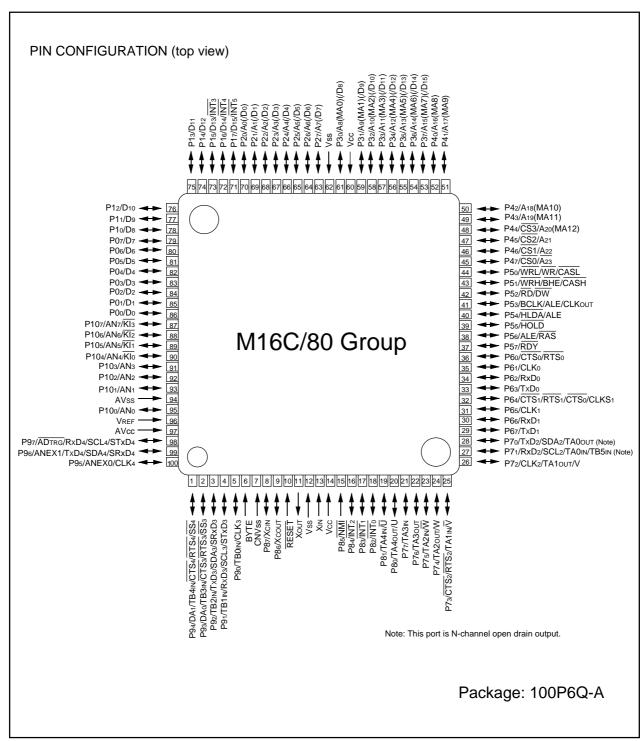
Figure 1.1.2. Pin configuration for 100-pin version (top view) (2)
