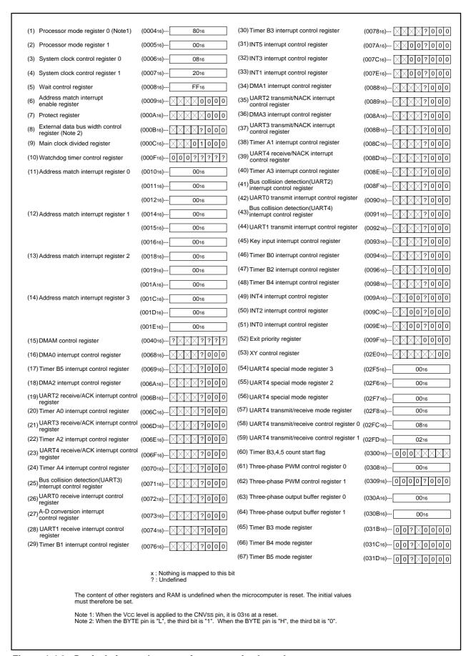
Figure 1.4.3. Device's internal status after a reset is cleared
