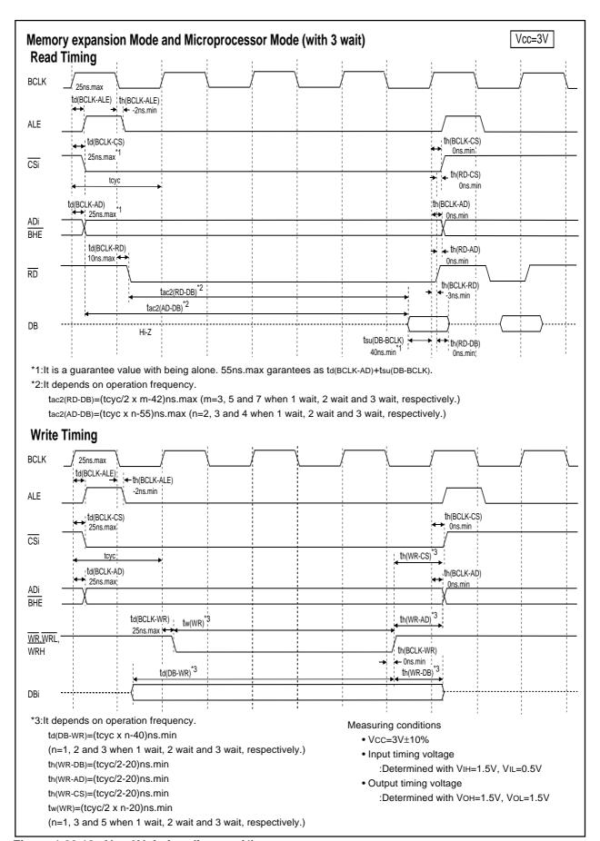
Figure 1.28.18. Vcc=3V timing diagram (4)
