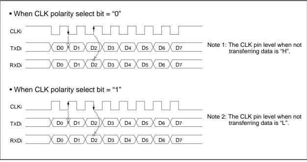
Figure 1.17.3. Polarity of transfer clock
