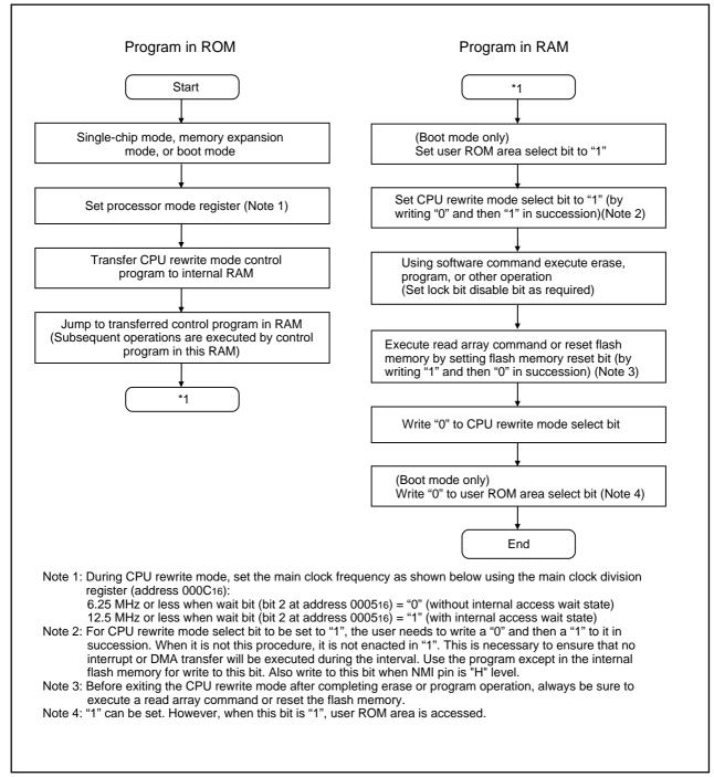
Figure 1.30.2. CPU rewrite mode set/reset flowchart
