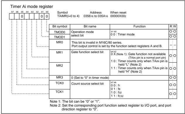
Figure 1.13.5. Timer Ai mode register in timer mode
