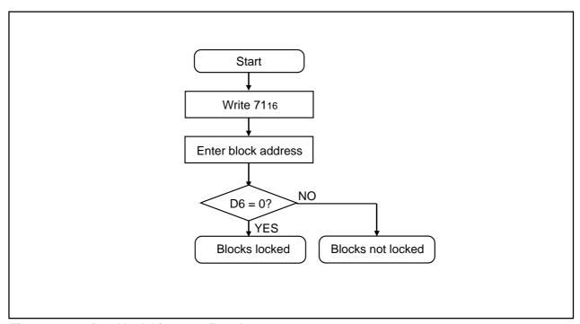
Figure 1.30.7. Read lock bit status flowchart
