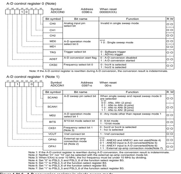
Figure 1.21.6. A-D conversion register in single sweep mode
