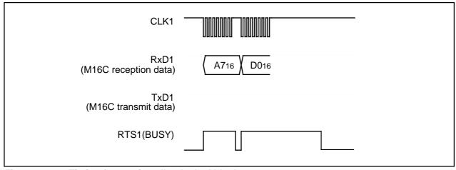
Figure 1.31.9. Timing for erasing all unlocked blocks
