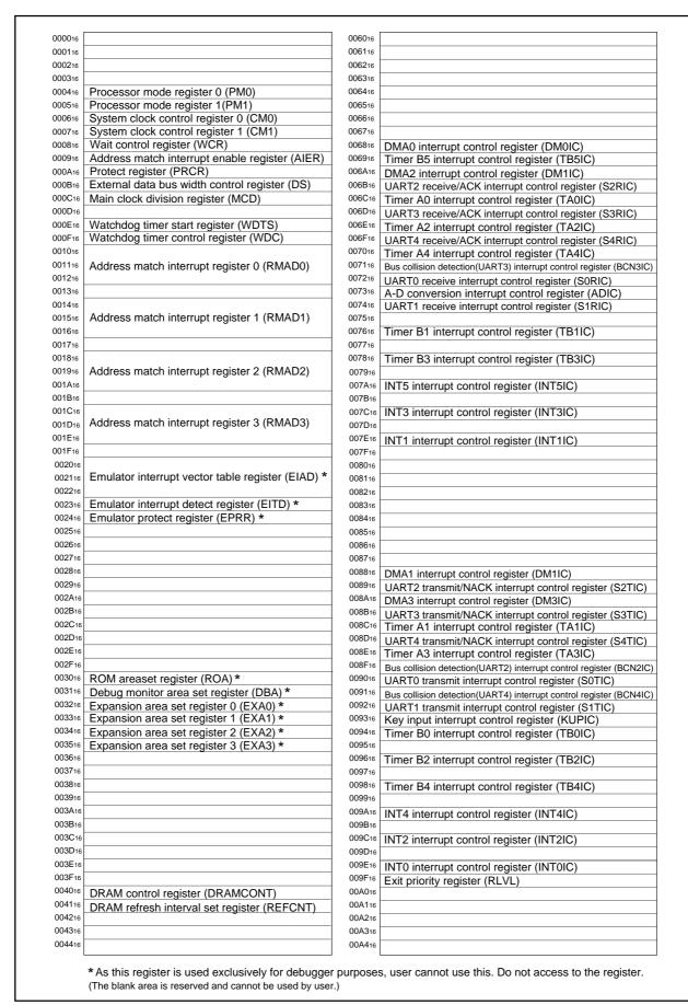
Figure 1.5.1. Location of peripheral unit control registers (1)
