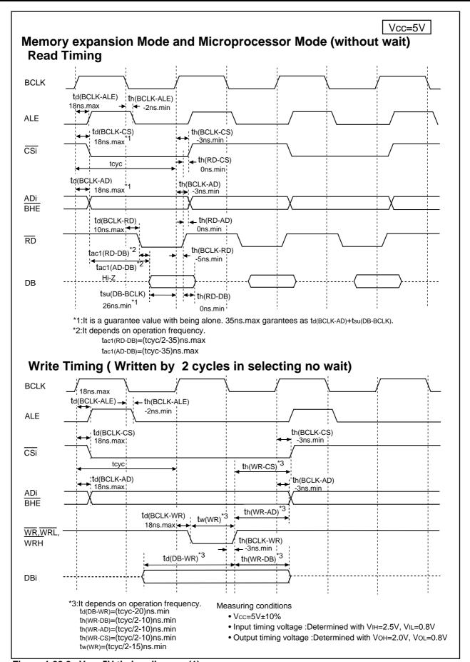
Figure 1.28.2. Vcc=5V timing diagram (1)
