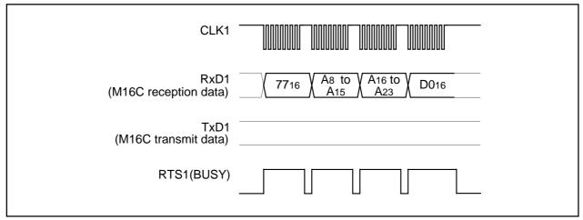
Figure 1.31.10. Timing for the lock bit program
