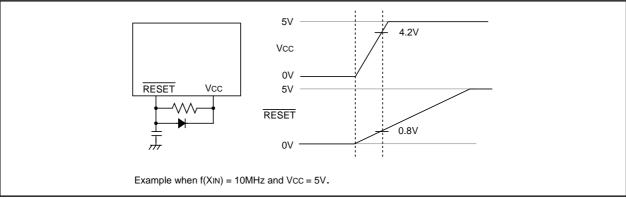
Figure 1.4.1. Example reset circuit
