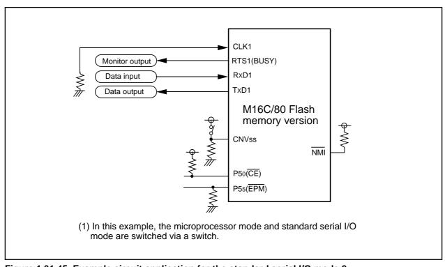
Figure 1.31.45. Example circuit application for the standard serial I/O mode 2
