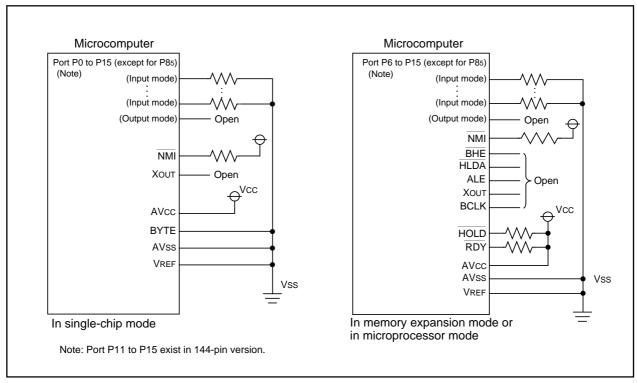
Figure 1.26.16. Example connection of unused pins
