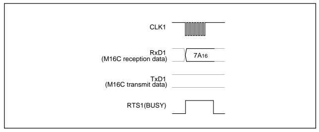
Figure 1.31.12. Timing for enabling the lock bit
