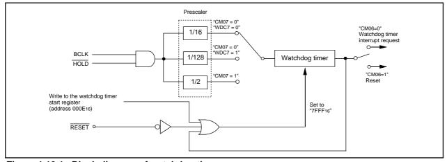
Figure 1.10.1. Block diagram of watchdog timer
