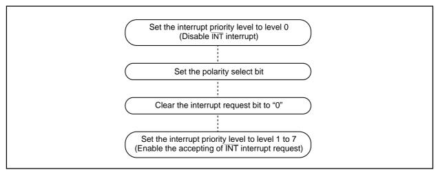
Figure 1.27.2. Switching condition of INT interrupt request
