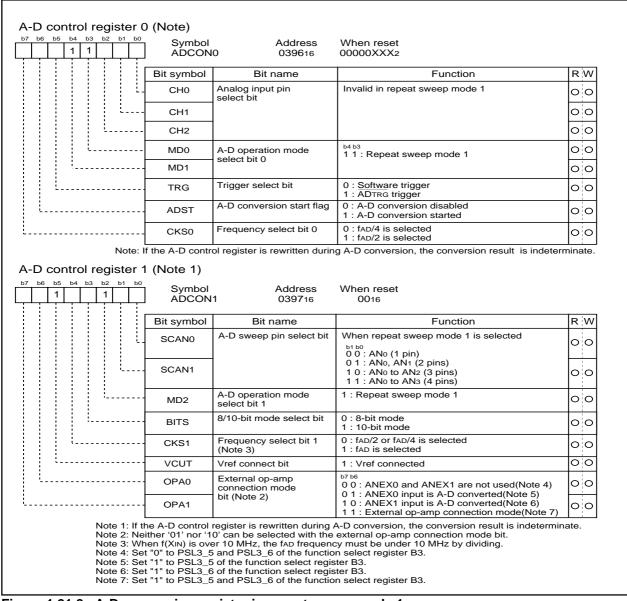
Figure 1.21.8. A-D conversion register in repeat sweep mode 1
