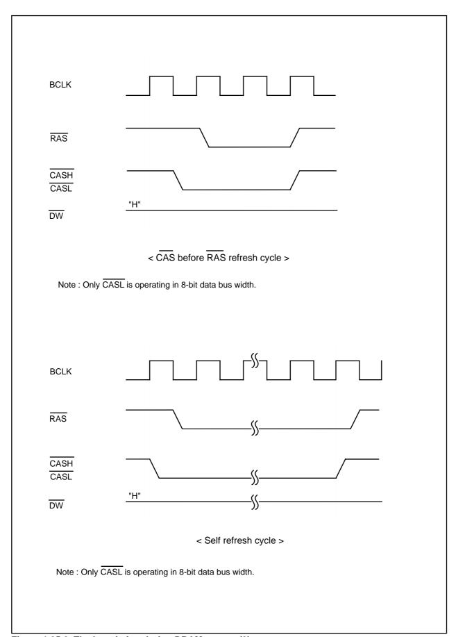
Figure 1.25.6. The bus timing during DRAM access (3)
