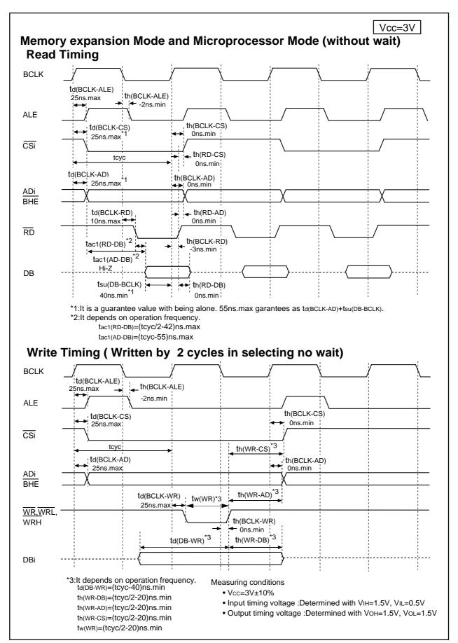
Figure 1.28.15. Vcc=3V timing diagram (1)
