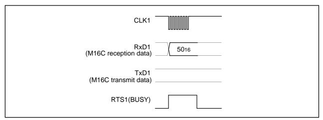
Figure 1.31.6. Timing for clearing the status register
