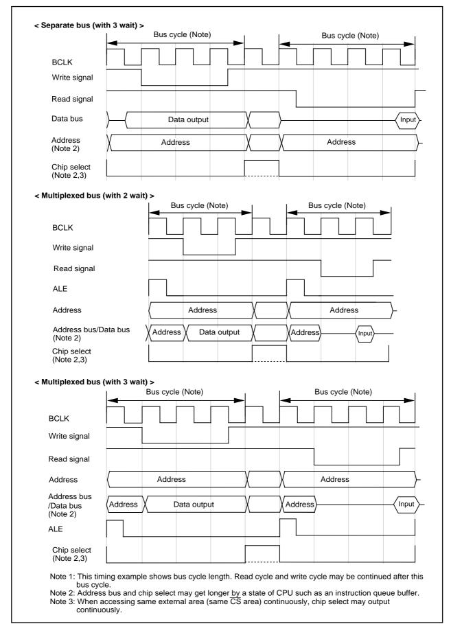
Figure 1.7.8. Typical bus timings using software wait
