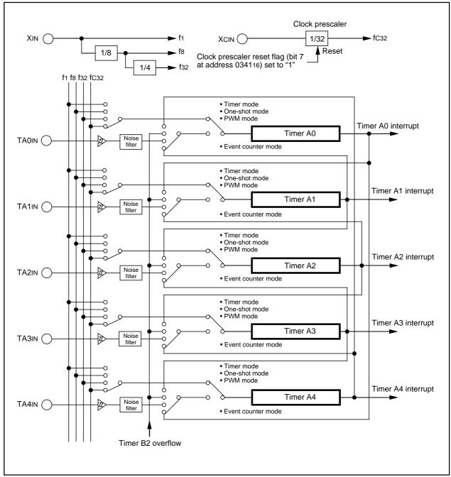
Figure 1.12.1. Timer A block diagram
