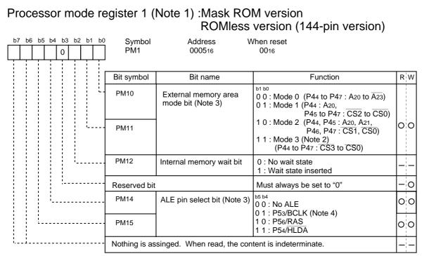
Note 1: Set bit 1 of the protect register (address 000A<sub>16</sub>) to "1" when writing new values to this register.
