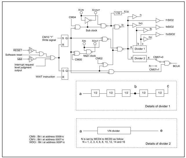
Figure 1.8.3. Clock generating circuit
