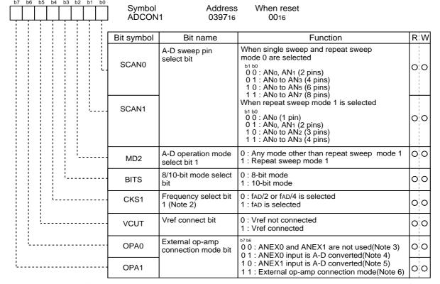
Note 1: If the A-D control register is rewritten during A-D conversion, the conversion result is indeterminate.
