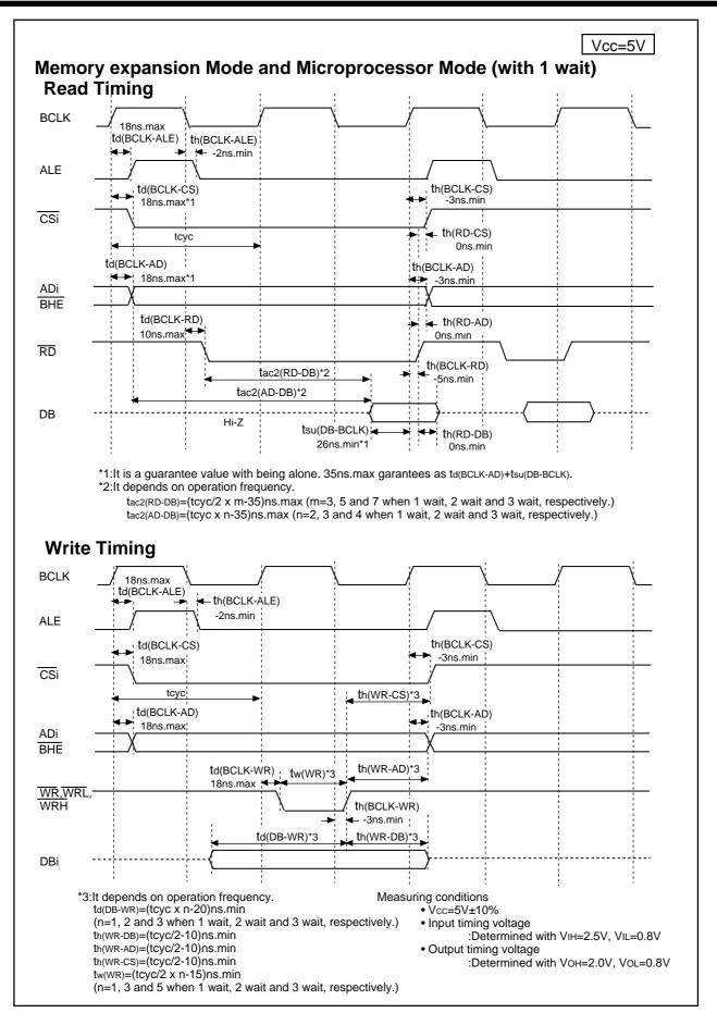
Figure 1.28.3. Vcc=5V timing diagram (2)
