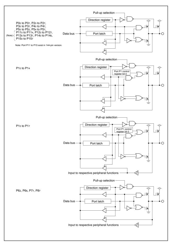
Figure 1.26.1. Programmable I/O ports (1)
