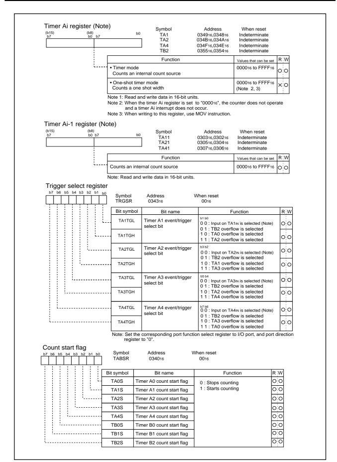
Figure 1.15.3. Registers related to timers for three-phase motor control
