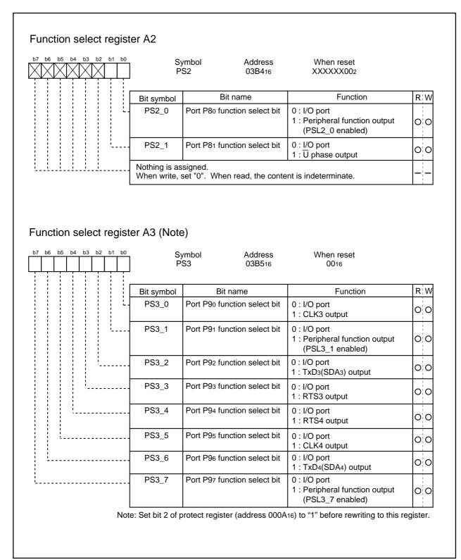
Figure 1.26.9. Function select register A (2)
