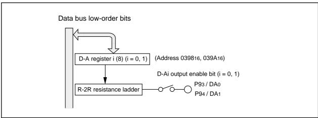
Figure 1.22.1. Block diagram of D-A converter
