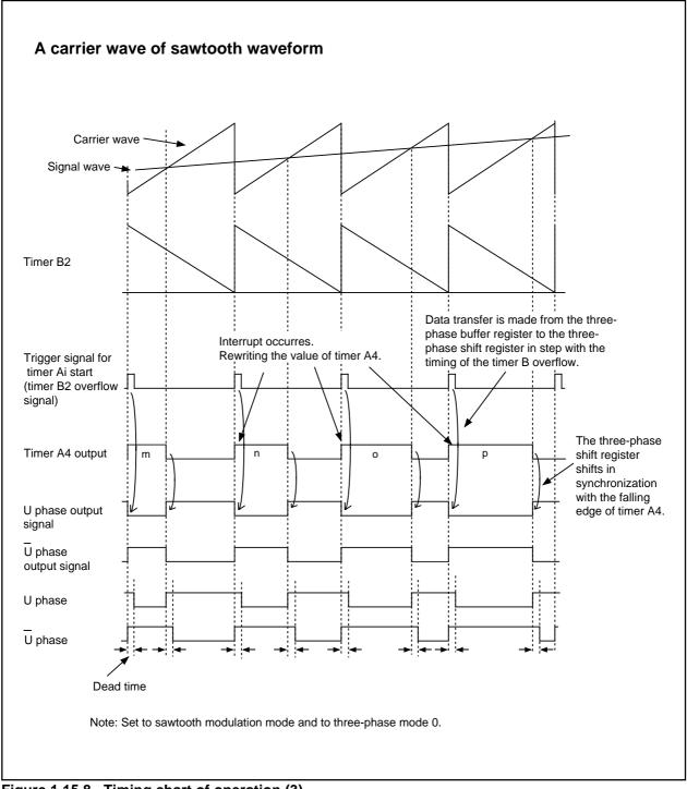
Figure 1.15.8. Timing chart of operation (3)
