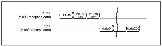
Figure 1.31.36. Timing for boot ROM area output
