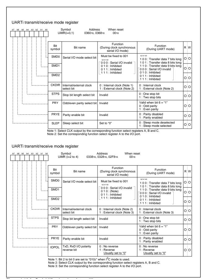
Figure 1.16.6. Serial I/O-related registers (2)
