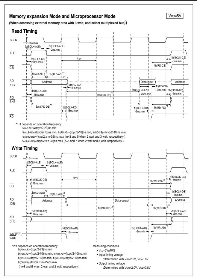
Figure 1.28.7. Vcc=5V timing diagram (6)
