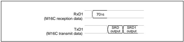
Figure 1.31.25. Timing for reading the status register
