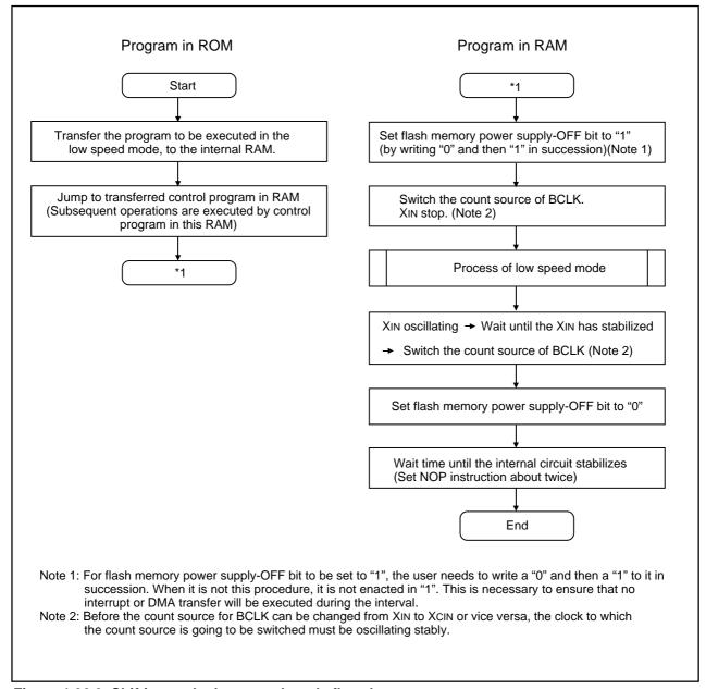
Figure 1.30.3. Shifting to the low speed mode flowchart
