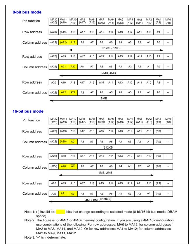
Figure 1.25.2. Output format for multiplexed addresses
