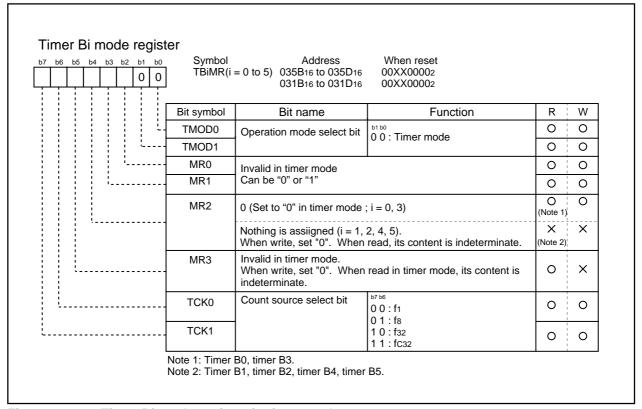
Figure 1.14.4. Timer Bi mode register in timer mode
