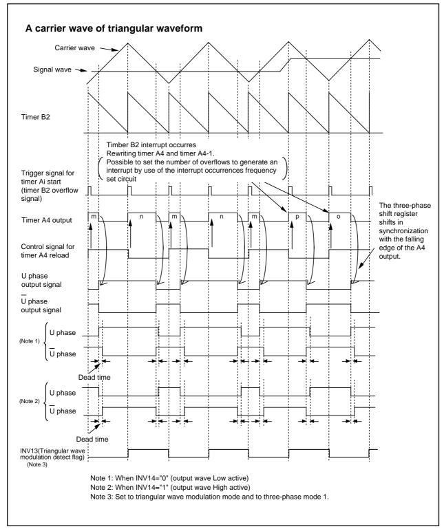
Figure 1.15.6. Timing chart of operation (1)
