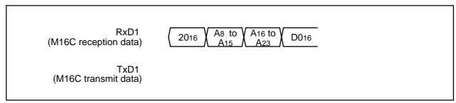
Figure 1.31.28. Timing for block erasing
