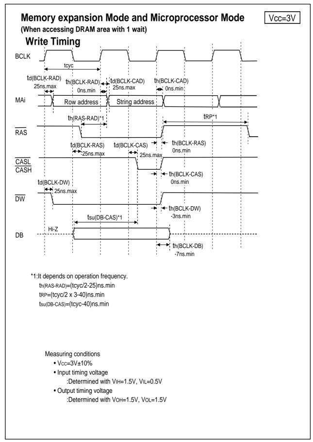
Figure 1.28.22. Vcc=3V timing diagram (8)
