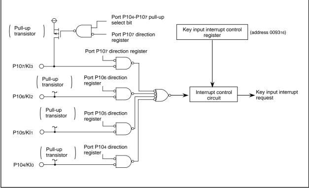
Figure 1.9.10. Block diagram of key input interrupt
