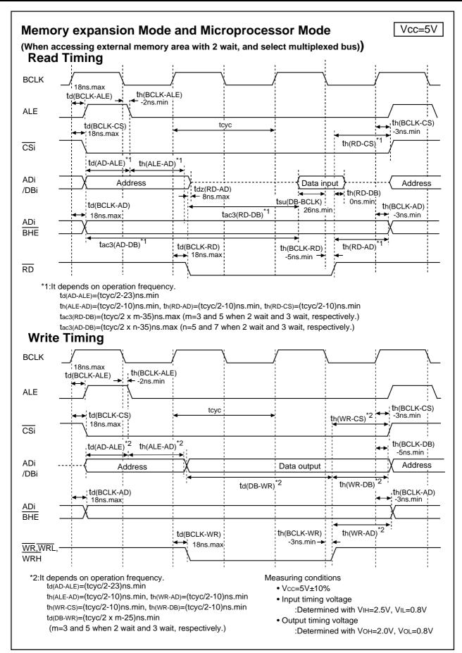
Figure 1.28.6. Vcc=5V timing diagram (5)
