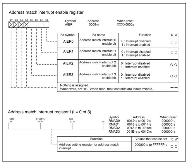
Figure 1.9.11. Address match interrupt-related registers
