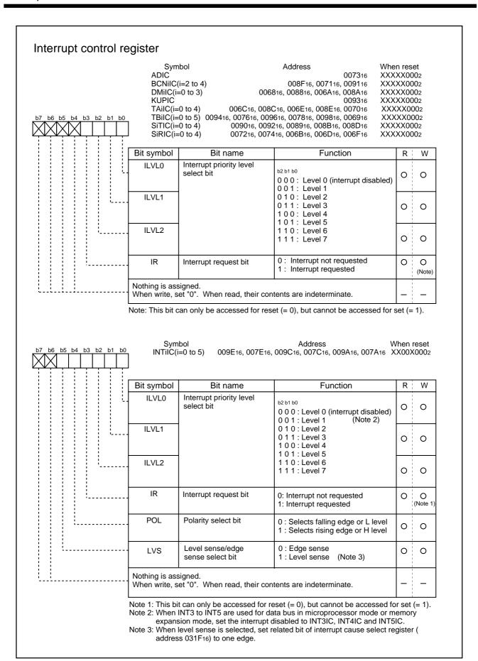
Figure 1.9.3. Interrupt control register
