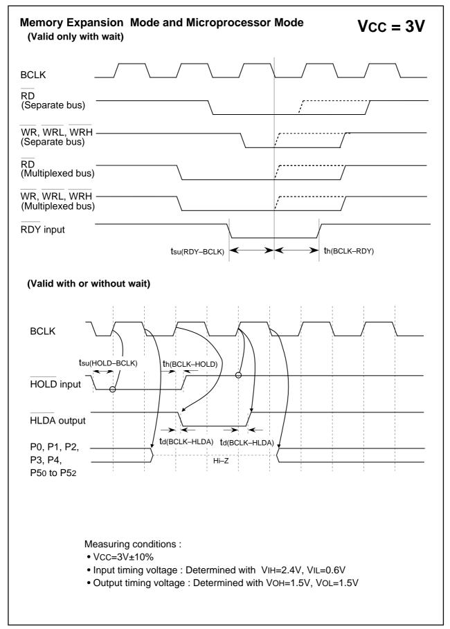
Figure 1.28.27. Vcc=3V timing diagram (13)
