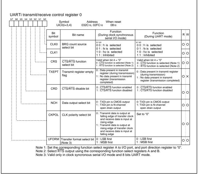
Figure 1.16.8. Serial I/O-related registers (4)
