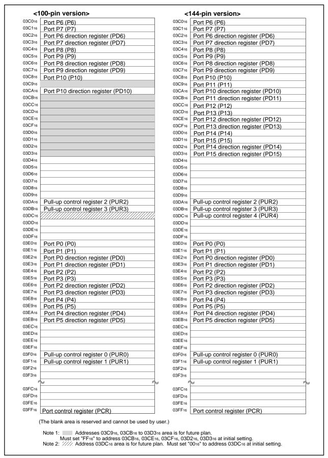
Figure 1.5.4. Location of peripheral unit control registers (4)
