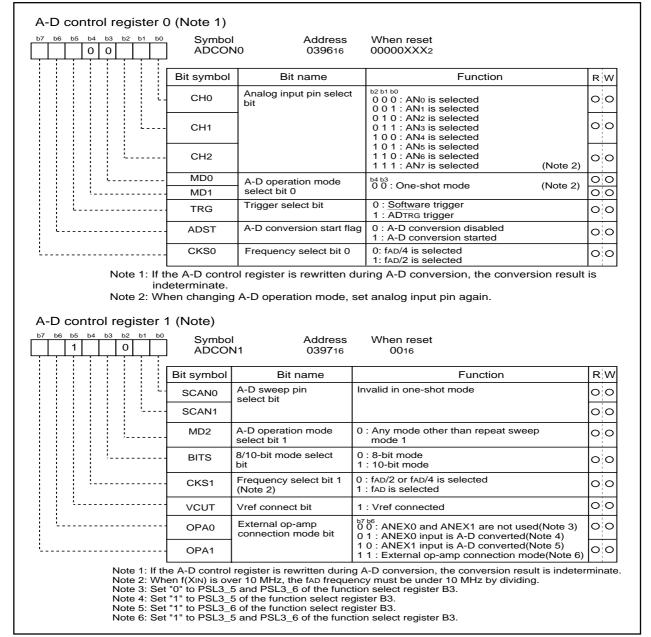
Figure 1.21.4. A-D conversion register in one-shot mode
