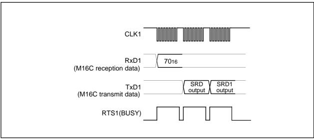
Figure 1.31.5. Timing for reading the status register
