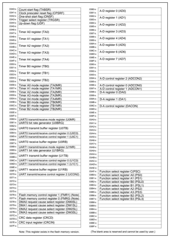
Figure 1.5.3. Location of peripheral unit control registers (3)
