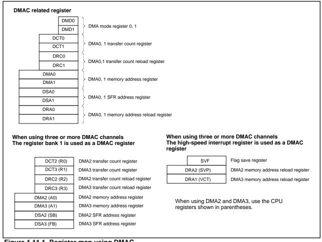
Figure 1.11.1. Register map using DMAC
