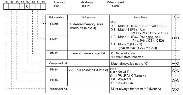
Note 1: Set bit 1 of the protect register (address 000A<sub>16</sub>) to "1" when writing new values to this register.
