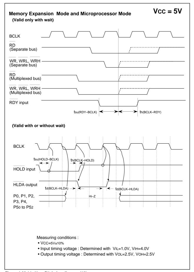
Figure 1.28.14. Vcc=5V timing diagram (13)
