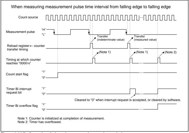
Figure 1.14.7. Operation timing when measuring a pulse period
