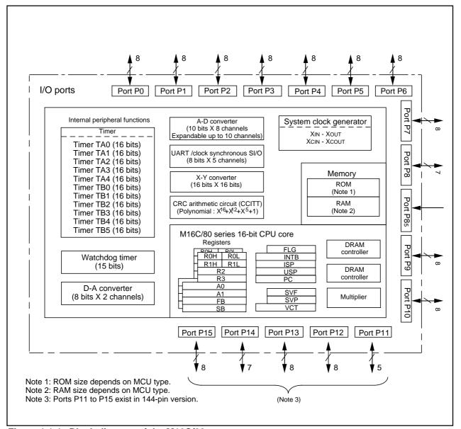
Figure 1.1.4. Block diagram of the M16C/80 group
