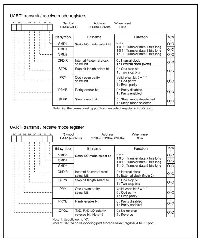
Figure 1.18.1. UARTi transmit/receive mode register in UART mode
