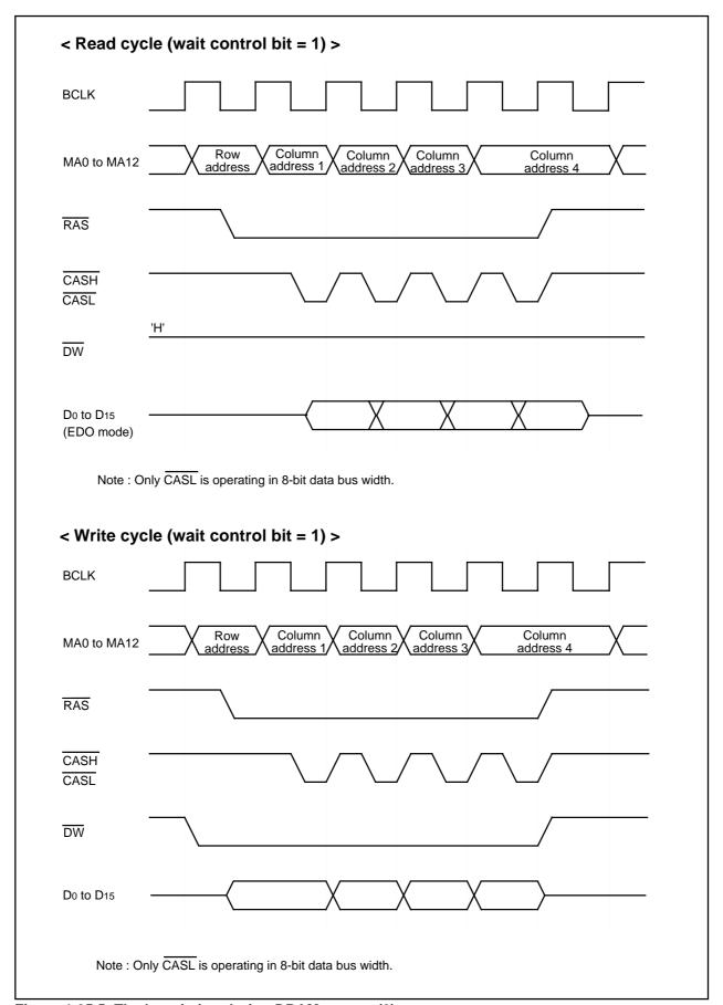
Figure 1.25.5. The bus timing during DRAM access (2)
