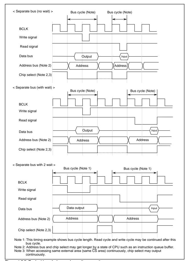
Figure 1.7.7. Typical bus timings using software wait
