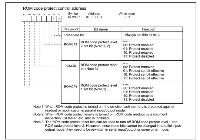
Figure 1.30.9. ROM code protect control address
