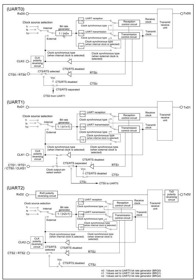
Figure 1.16.1. Block diagram of UARTi (i = 0 to 2)
