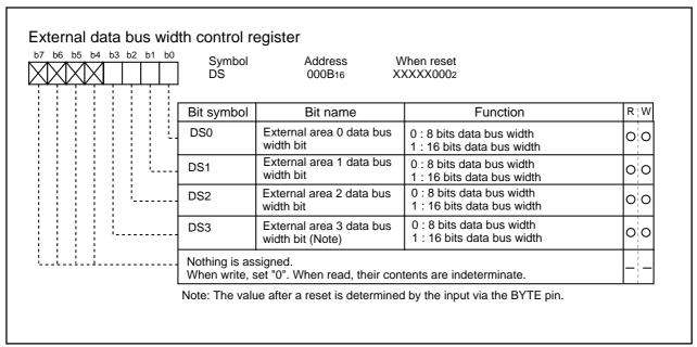
Figure 1.7.1. External data bus width control register
