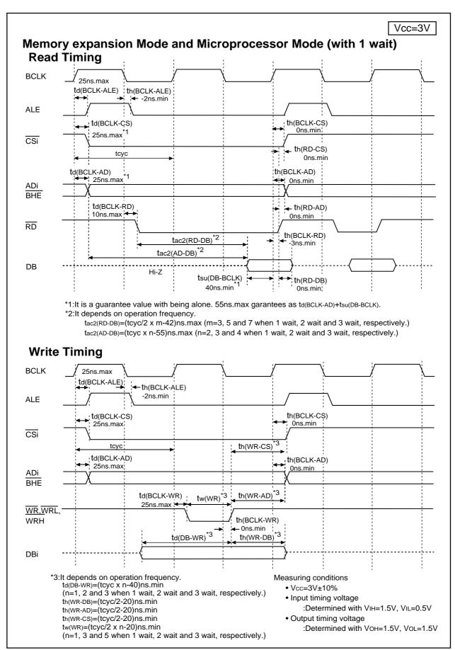
Figure 1.28.16. Vcc=3V timing diagram (2)
