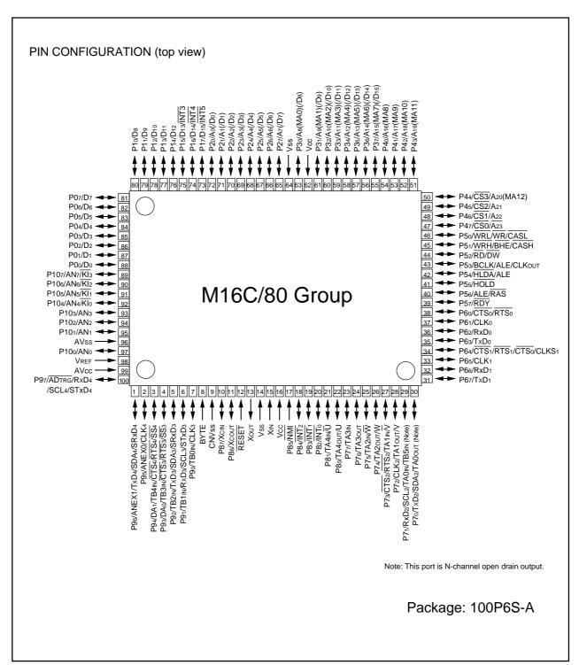
Figure 1.1.1. Pin configuration for 100-pin version (top view) (1)
